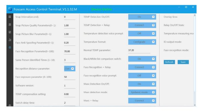
**Snap Interval:** set the face capture time interval to avoid repeated capture of pictures in a short time. **Face Anti-Spoofing Parameter**: Set the Face Anti-Spoofing Parameter, 0-1, the larger the value, the stricter the living body detection and the safer it is.
